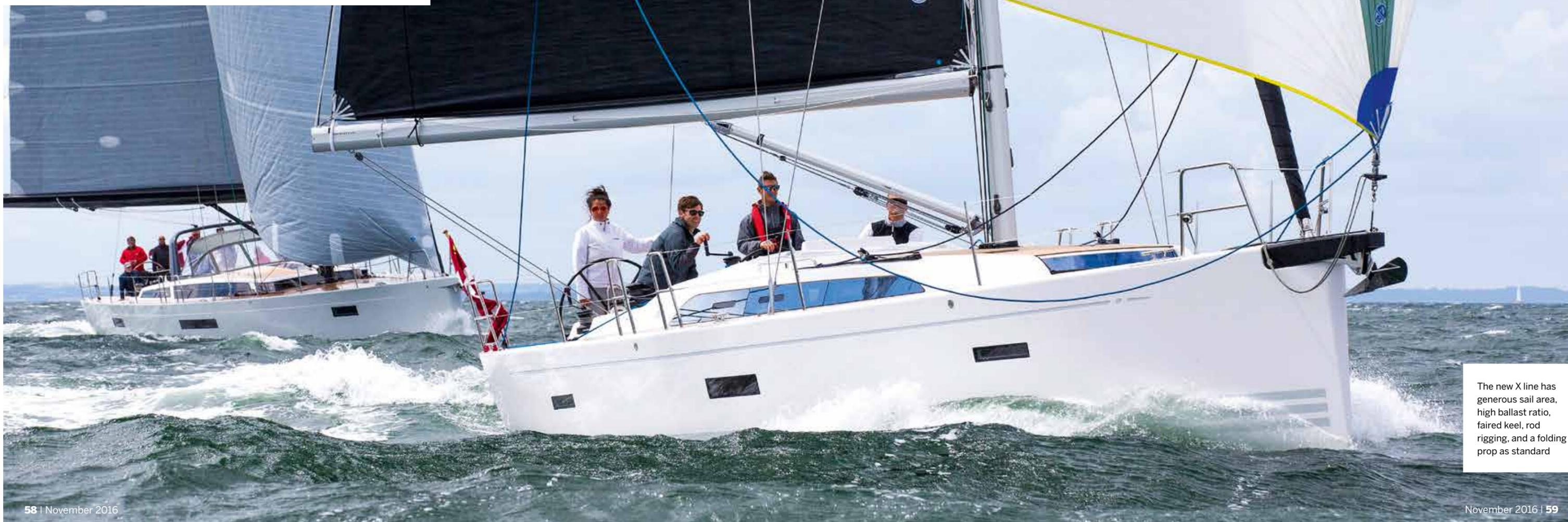
The new X line has generous sail area, high ballast ratio, faired keel, rod rigging, and a folding prop as standard
