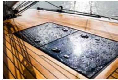
**Above:** Flush, frameless hatches create a feeling of uninterrupted flow across the deck
