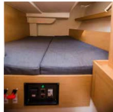
the best use of the layout. The forward-looking coachroof window is a stylish touch to go with the hull portlights and the large deck hatch. Headroom of 6ft 4in is carried up to the island berth, which is somewhat elevated with generous stowage beneath. The berth lifts on gas struts for easy access.
