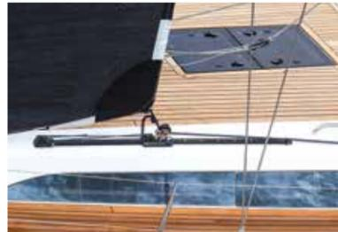
**Above:** The jib tracks are mounted inboard on the coachroof, which helps the X4 to point
